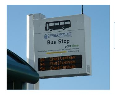
Electronic timetable display contained within the 'flag' at the top of a free standing bus stop post.
